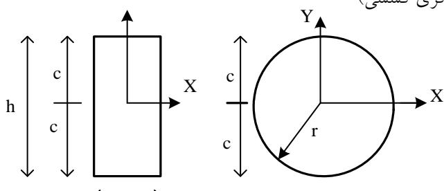
$$\sigma_{max} = \pm \frac{MC}{I} = \pm \frac{M}{S} \quad , \quad S = \frac{I}{C}$$
