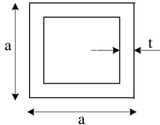
$$\alpha = \frac{\frac{\text{مقاومت پیچشی ۱}}{\text{مقاومت پیچشی ۲}}}{\frac{\tau_2}{\tau_1}} = \frac{\frac{\frac{\text{K}}{\sqrt{A_{m2}t_2}}}{\frac{\text{K}}{\sqrt{A_{m1}t_1}}}}{\frac{\tau_2}{\tau_1}} = \frac{\frac{A_{m1}t_1}{A_{m2}t_2}}{\frac{\tau_2}{\tau_1}} = \frac{\frac{2 \times 2 A_{m2} \times \frac{1}{2} t_2}{A_{m2} \times t_2}}{\frac{\tau_2}{\tau_1}} = 2$$
